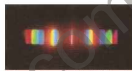
The spectrum of white light due to diffraction grating of 2000 slits.
