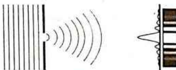
Fig.9.11(b): A diffraction pattern due to bending of light through edges of a narrow slit.
