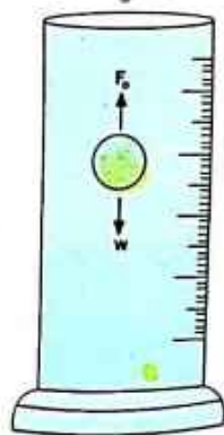
Fig.6.3: Two opposite forces acting on a body moving through a viscous medium
