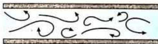
Fig.6.7: Turbulent or Irregular flow
