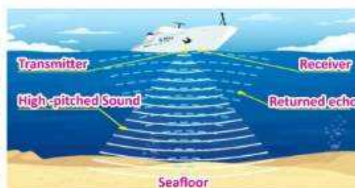
Fig. 13.15: Illustration of sonar used by a ship.
