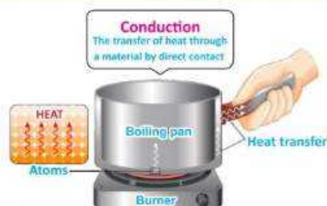
Fig. 11.14: Heat transfer through conduction in a boiling pan
