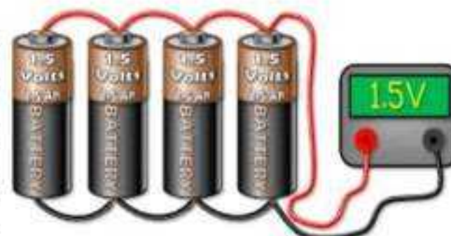
Fig. 16.9: Four 1.5 V batteries connected in parallel
