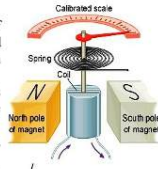
Figure 18.12 schematic diagram of Galvanometer
