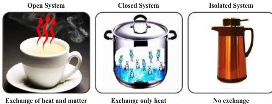
Figure 16.4 Open, Close and Isolated system
