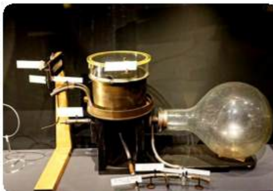
Figure 28.9 Wilson cloud Chambers
