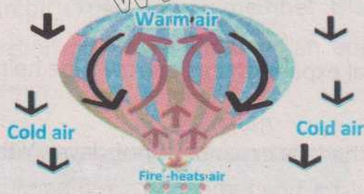
Fig. 10.6: When hot air balloon is heated, air inside the balloon expands and becomes less dense, causing the balloon to rise
