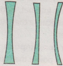
Double concave Plano-concave Convexo-concave
