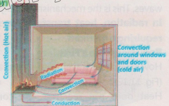
Fig. 11.8: Heating room by convection
