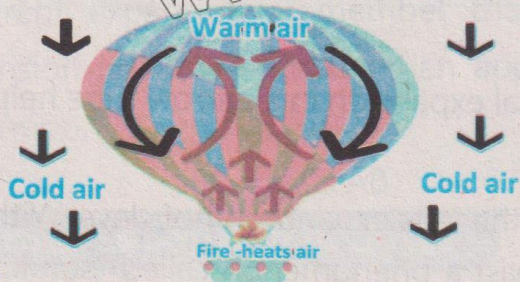
Fig. 10.6: When hot air balloon is heated, air inside the balloon expands and becomes less dense, causing the balloon to rise
