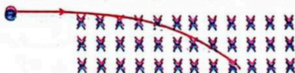
Fig.13.16(b) The electron is deflected downward under the action of magnetic force.
