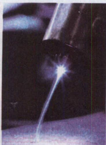
Welding Arc Plasma
