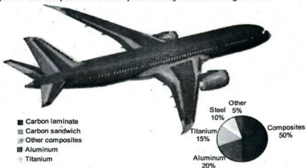
Fig. 7.32: Composition of airplane's body
