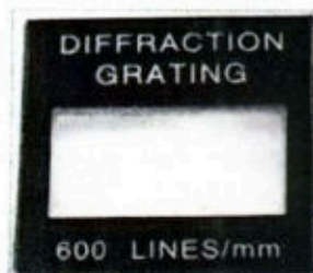
Figure 18.9 (a): Diffraction Grating
