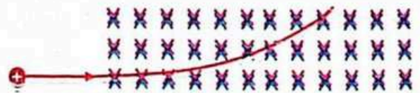
Fig.13.16(a) The proton is deflected upward under the action of magnetic force.
