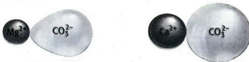
Fig 5.4 Magnesium ions are better polarisers of carbonate ions than calcium ions.
