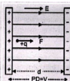
Figure 10.10 (b): Charged Particle in an electric field.
