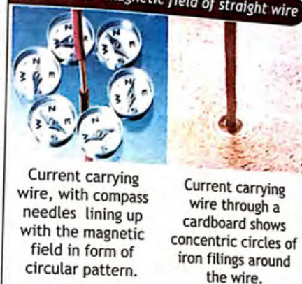
Figure 15.2 - Magnetic field of straight wire
