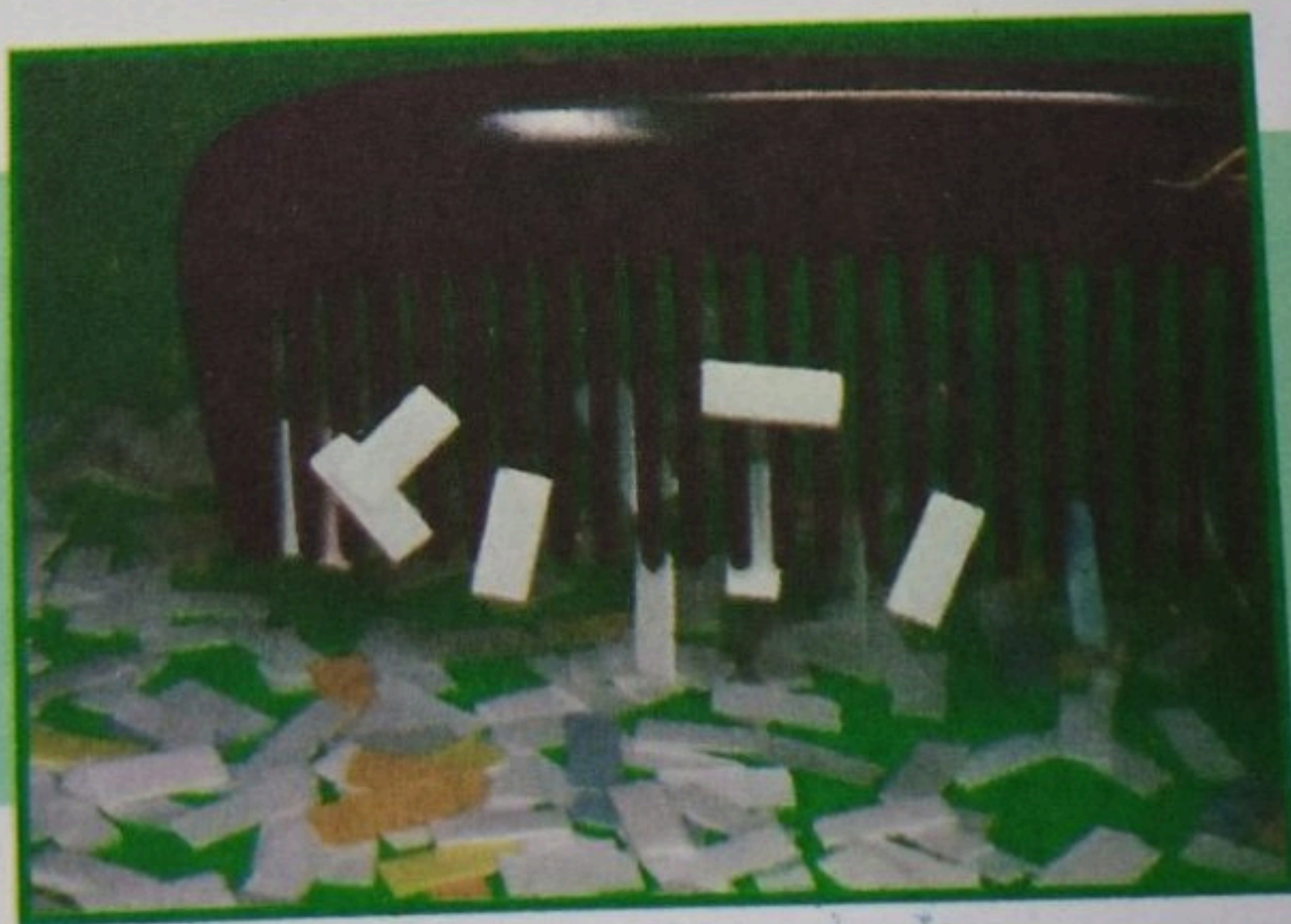
Fig:63 Using static charge to pick up pieces of paper with a comb.
