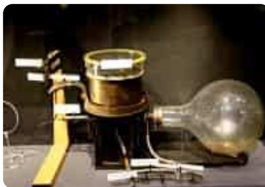
Figure 28.9 Wilson cloud Chambers
