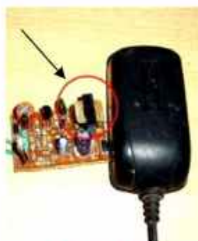
Fig: 16.21 Transformer battery charger
