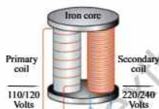
Fig: 16.18 (a) Step up transformer
