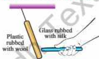
Fig: 14.4 (c) Glass rod attracts plastic rod
