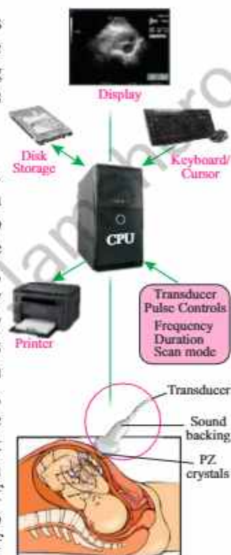
Fig: 11.14. The schematic diagram of the ultrasound scan machine
