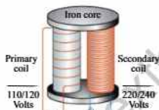
Fig: 16.18 (a) Step up transformer
