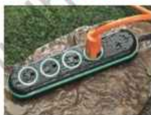
Fig: 15.24 Electrical extension placed damped environment
