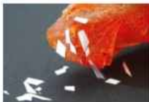
Fig: 14.3 The amber rubbed with silk attracts small pieces of paper
