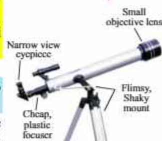
Fig: 13.25. Mechanical parts of a refracting telescope
