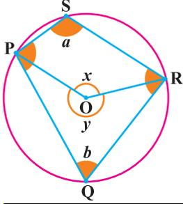
عمل:  $m\angle Q + m\angle S = 180^\circ$
